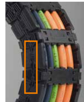
Elastic spring elements as vibration-dampening fasteners for chain links.
