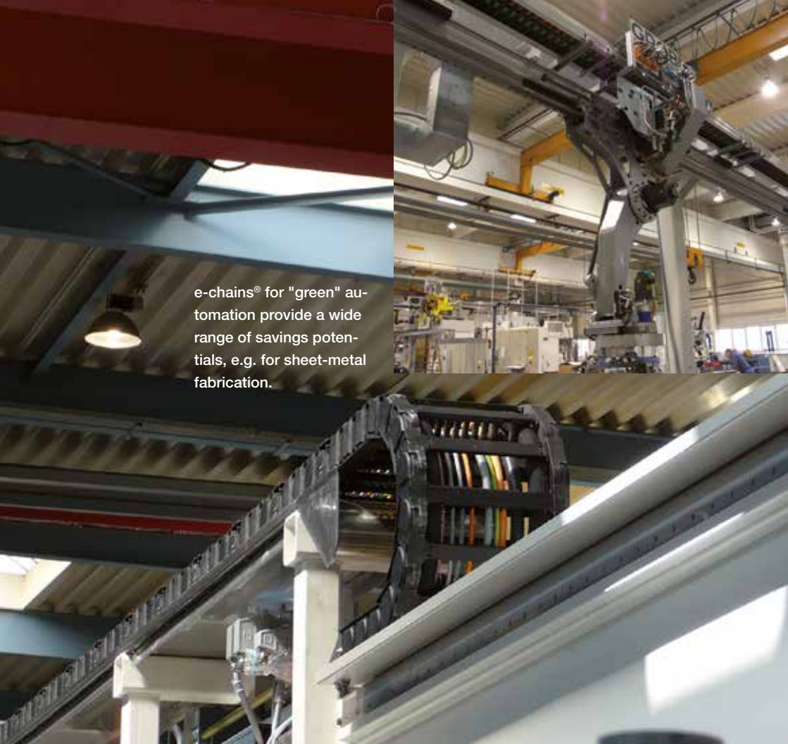
Energy-efficient e-chainsystem® P4 – rolling instead of gliding.
